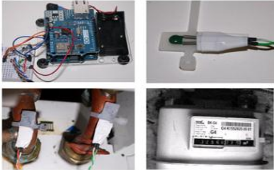
Figure 2. Prototype System including Arduino (top left), temperature sensors (top right), sensors affixed to pipes (bottom left), and feed from gas meter camera (bottom right).
